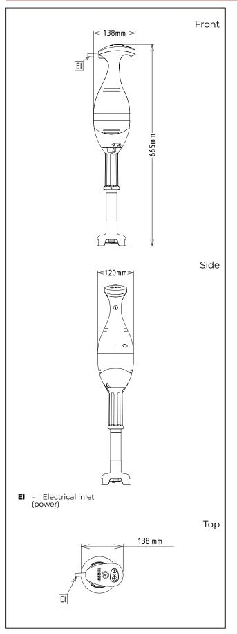
Electric Supply voltage: 220-240 V/1 ph/50/60 Hz **Electrical power max.:** 0.75 kW 0.75 kW **Total Watts:** Capacity: Capacity (up to): 80 Litre Key Information: External dimensions, Width: 138 mm External dimensions, 120 mm Depth: External dimensions, Height: 665 mm **Shipping weight:** 4.2 kg
